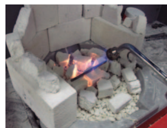
Year 10 Screwdriver blade heat treatment on the brazing hearth and forge
